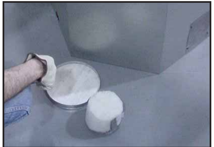
Figure 9.11 Discard the seal cap, remove and discard the insulation basket. Note: Once the vent cap has been removed it CANNOT be reattached.
